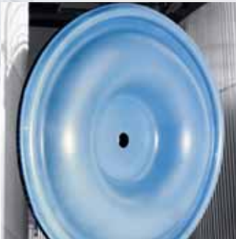
Diaphragm Before Metal Chip Test.
