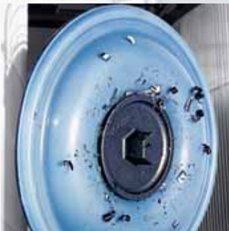
Diaphragm After Metal Chip Test.
